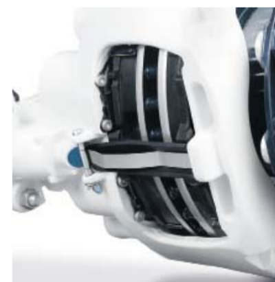
Figure 1: Permissible areas for edge ruptures are marked, but must be no more than 10% of the lining surface.
